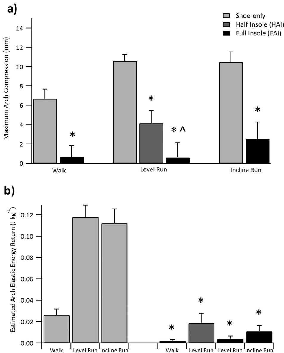
**Figure 1.** (a) Maximum arch compression (mm; mean  $\pm$  S.E.M.) relative to arch height at minimal shoe-only level running initial foot contact. (b) Estimated elastic energy ( $\text{J kg}^{-1}$ , mean  $\pm$  S.E.M.) returned from the arch of the foot in one step. \*indicates significantly different ( $p < 0.05$ ) to the minimal shoe-only trial in the same condition, ^ indicates significant difference between the half arch insole (HAI) and full arch insole (FAI) (level running only).
